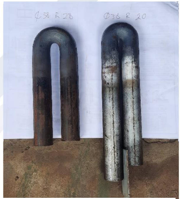
(U-Bend bending fabrication R20 mm & R 28 mm)
