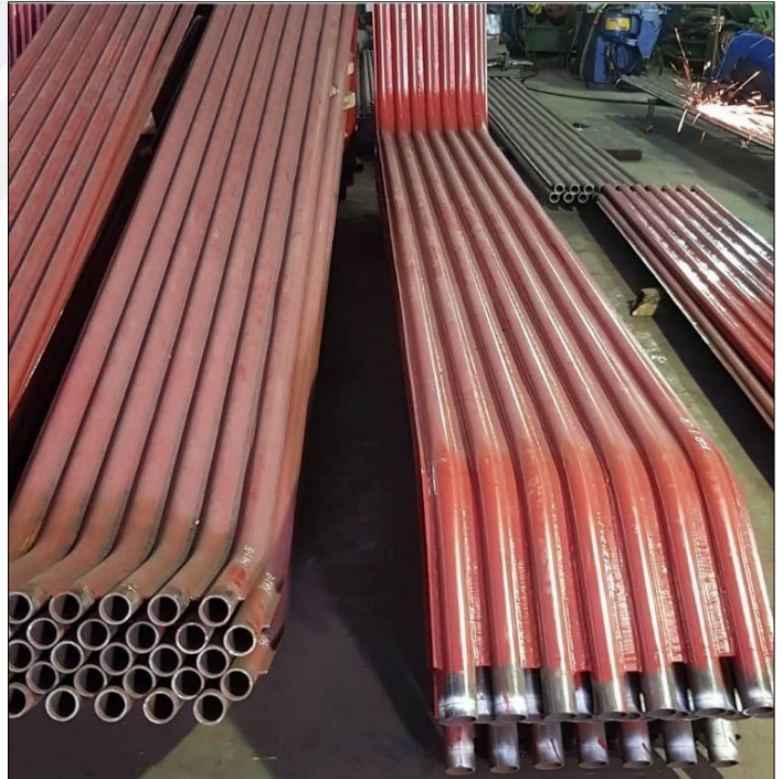
(Side & Right Wall Panel Tube Boiler)
