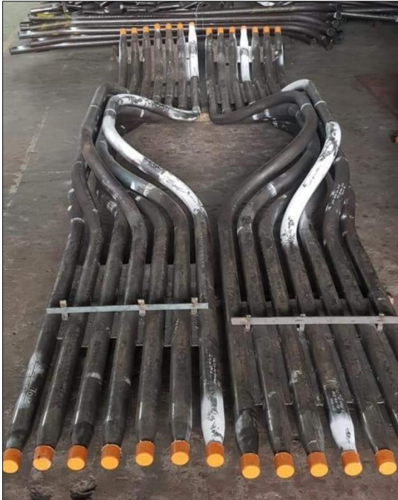
(Opening Tube Boiler)
