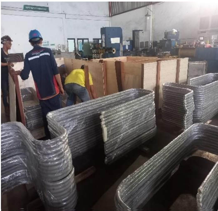
(PKT Kaltim 5 Pigtail Inlet Fabrication)
